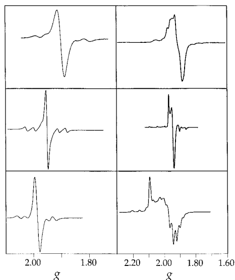
Figure 3. Room temperature (left) and 77 K frozen solution (right) X-band EPR spectra of [\text{MoOF}_5]^{2-} (top), [\text{MoOCl}_4(\text{H}_2\text{O})]^- (middle), and [\text{MoOBr}_5]^{2-} (bottom).
